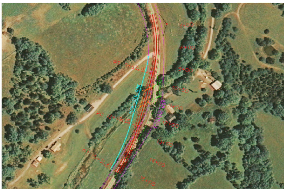
Figure 25: Proposed Realignment for Bridge #037B00023N
